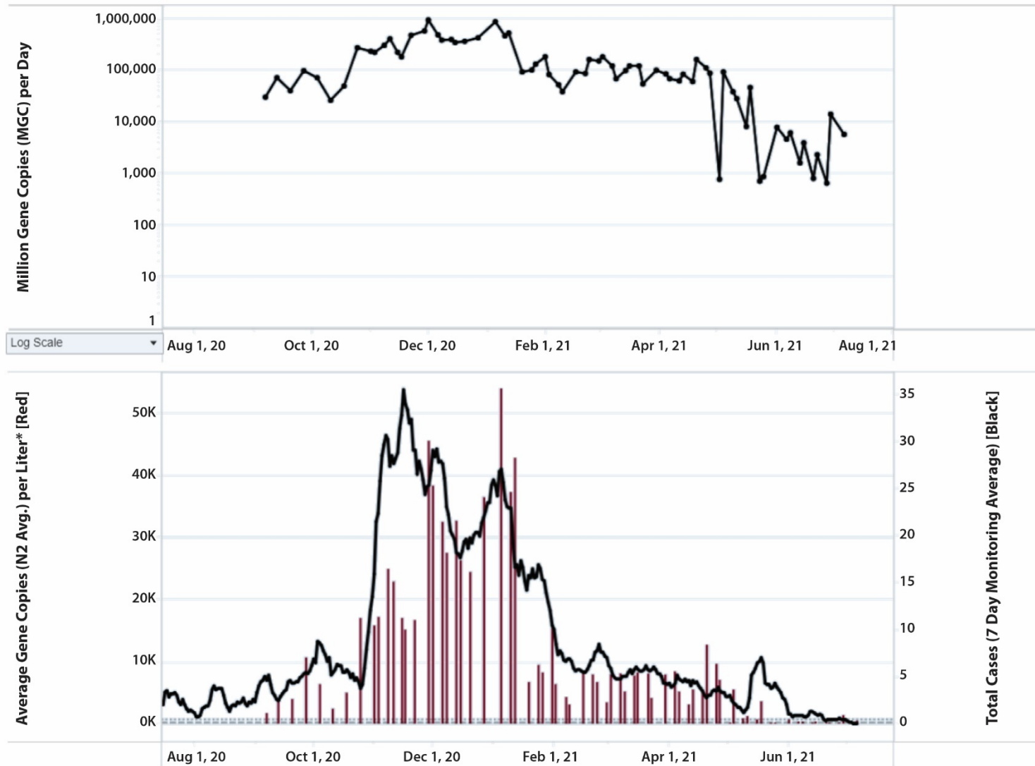
Figure 17. Ohio Coronavirus Wastewater Monitoring Network Dashboard showing city-specific results normalized by WWTP influent flow rate (top graph) and compared to the number of COVID-19 cases from individual testing (bottom graph) (Ohio DOH, 2020).
