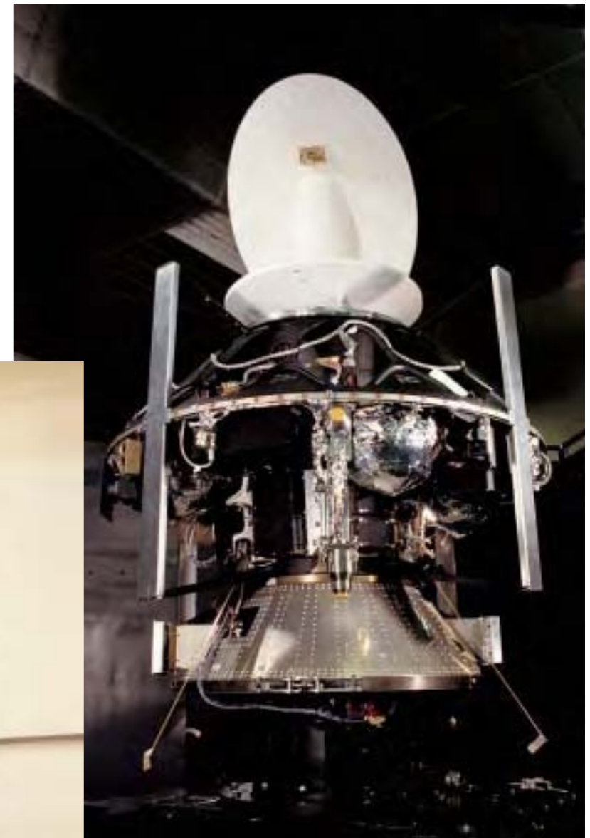
Sirio-2 complete, with the solar array panels removed.
