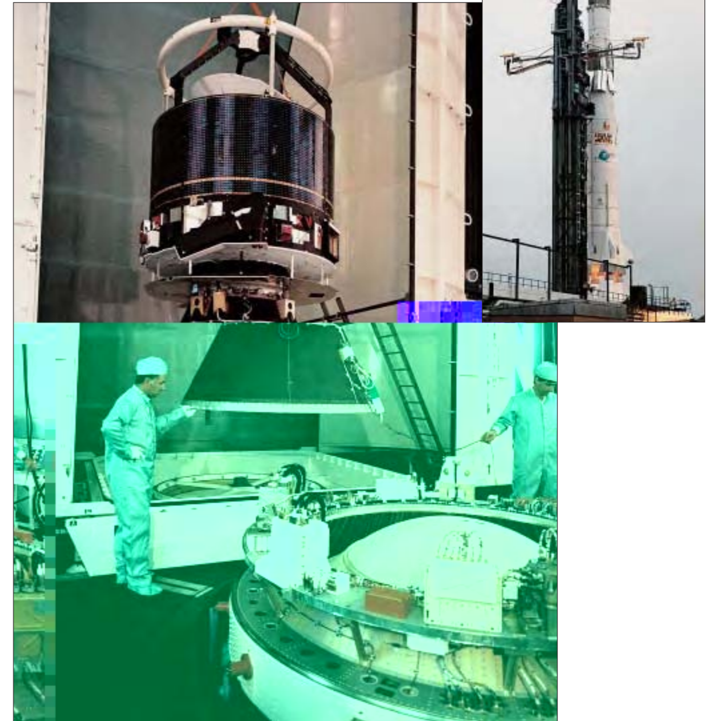
Installation of Giotto on its Ariane launcher at Kourou. The dome cover of Ariane's third stage liquid hydrogen tank can be seen protruding through the centre of the Vehicle Equipment Bay. (CSG/CNES/Arianespace)
