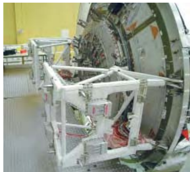
The External Payload Facility is installed on Columbus. Note the bolted cover over the module opening used during assembly.
