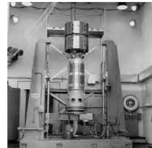
Right: ESRO-2 and its Scout stage 4 undergoing spin-balancing at the Western Test Range.
