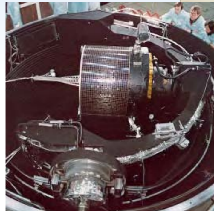
ISEE-2 installation in the HBF 3 facility at ESTEC for thermal-vacuum testing.
