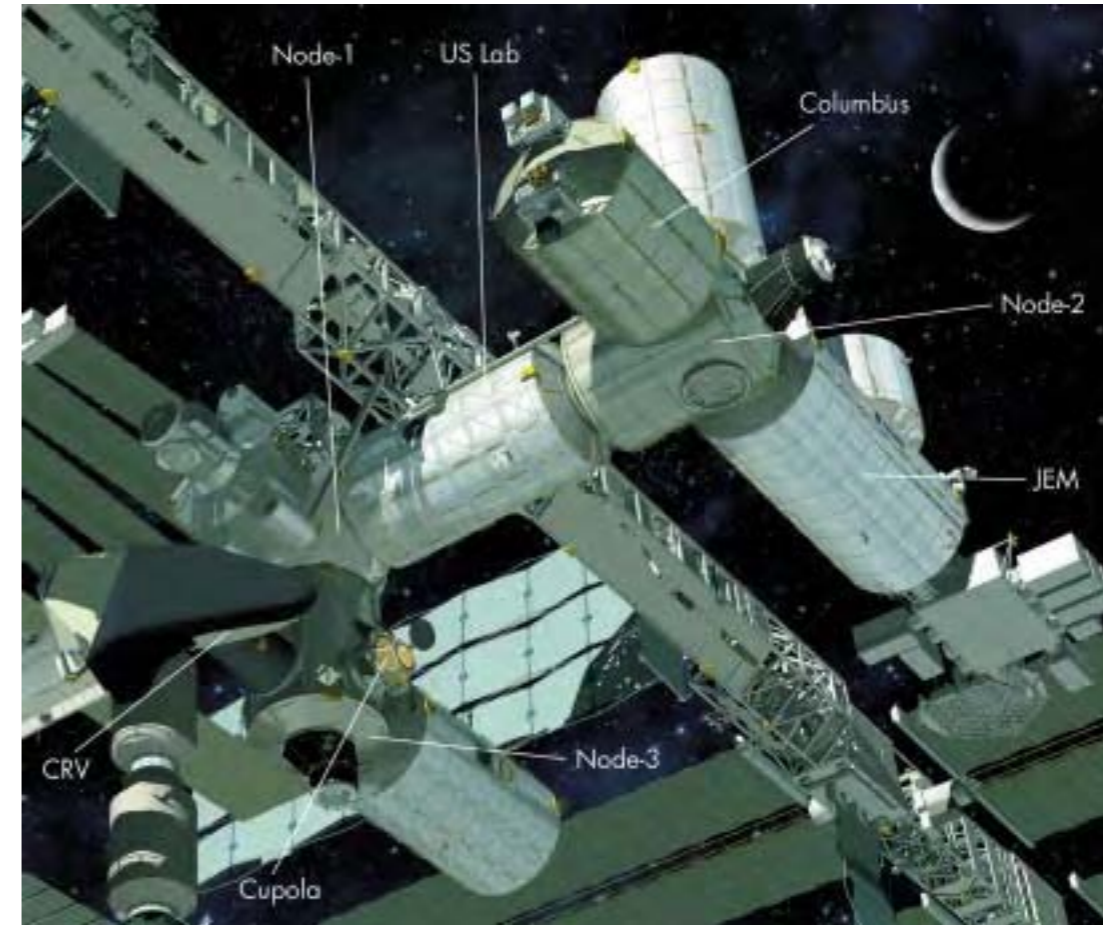
Top: the locations of Nodes-2/3. (CRV was the Crew Return Vehicle, cancelled by NASA in 2001.) Bottom: Node-2 arrives in the Space Station Integration Facility at KSC, June 2002.
