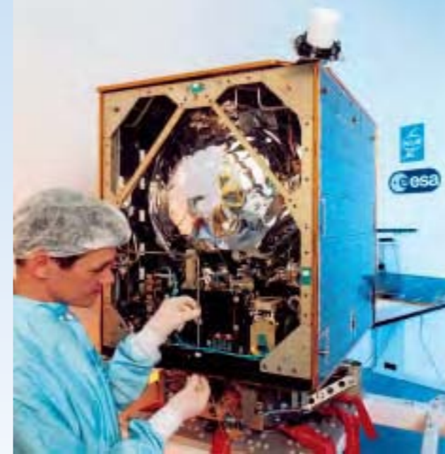
Above: completion of Sloshtsat. The 'spots' on the tank are some of the 270 platinum capacitors for measuring the thickness of water on the wall. Right: Sloshtsat being prepared for thermal-vacuum testing.
