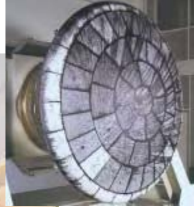
Main image: ARD integrated at Aerospatiale, Bordeaux. The heatshield included samples of new materials. Inset: post-flight measurements showed that the main shield was eroded by only 0.1-0.3 mm.
