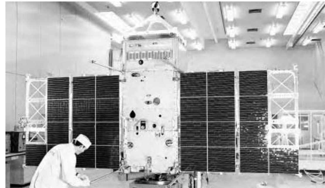
TD-1 in the integration hall at ESTEC, July 1971. The attitude control system held this side square on to the Sun.
