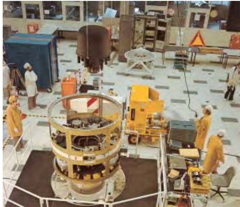
Integration of the Cos-B detector package and spacecraft prototypes at MBB.
