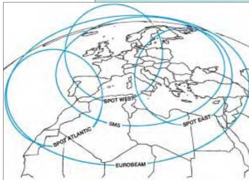
ECS-1 provided services to Europe and north Africa via three spot beams and a single Eurobeam. Its successors added the Satellite Multiservice System for business users.
