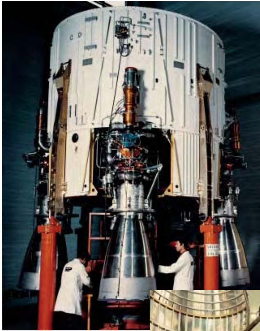
The engine bay of Ariane's first stage carried four Viking 5 engines. (Snecma Moteurs)
