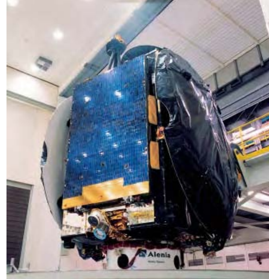
Artemis ready to be installed on its launcher. Note the south-face ion thruster package below the solar wing.
