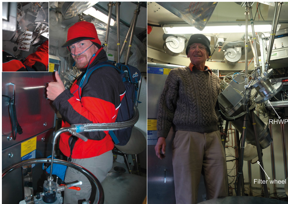
Figure 2. The image on the left shows APEX staff astronomer, Andreas Lundgren, in the process of refilling LABOCA. The transfer tube that is wrapped behind his back goes from a liquid helium dewar in the foreground to the helium tank in LABOCA, shown in the inset image in the upper left corner. The cryostat is shown from above in this inset. The image on the right shows Ernst Kreysa, the leader of the MPIfR bolometer group, together with the LABOCA cryostat in the Cassegrain cabin of the APEX telescope. At the time the picture was taken, the instrument PolKa was being installed.
