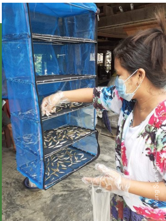
Low-cost, portable fish drier made from blue nylon netting, stainless steel wire and string with a zip
