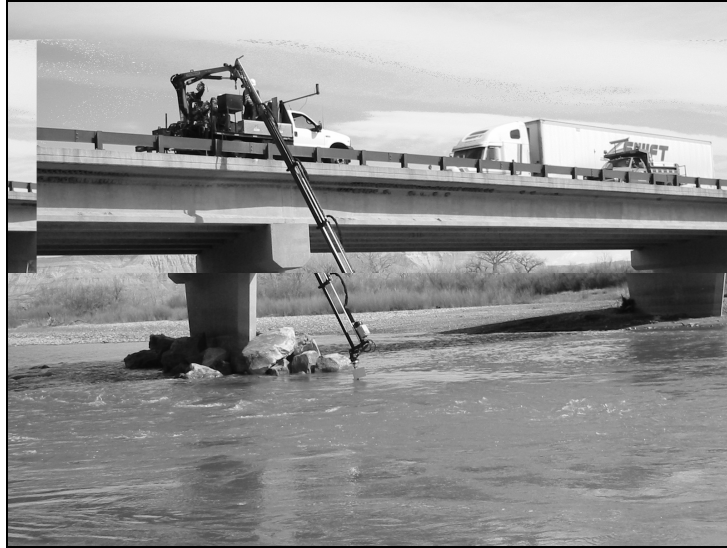
Figure 9.9. Sonar instrument deployed from articulated arm truck.
