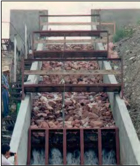
Figure 5.3. Test set up for 1994, d_{50} = 1.27 ft (386 mm).
