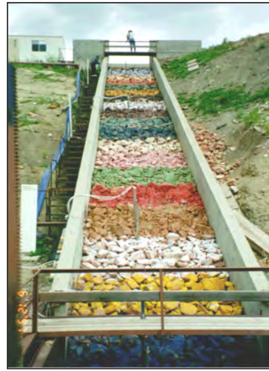
Figure 5.4. Test set up for 1997, d_{50} = 0.89 ft (271 mm).
