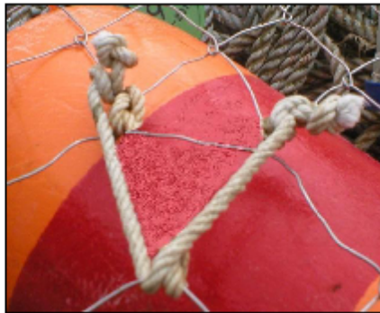
Biodegradable line holding closed an escape panel.
