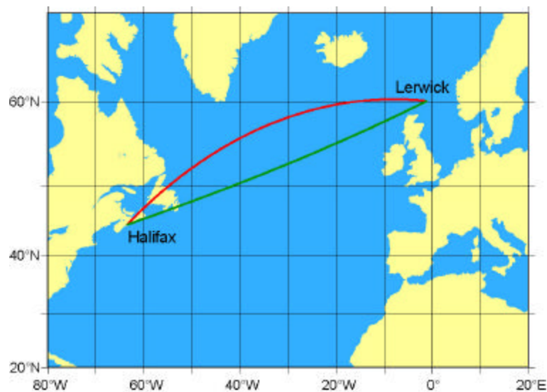
Figure 3.17 - Part of the North Atlantic Ocean on the Mercator Projection, showing great circle (curved) and rhumb-line (straight) paths between Halifax and Lerwick
