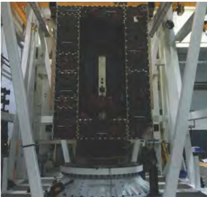
The rigid external structure of the GOES-R satellite, which will enclose the satellite's propulsion system and support the payloads, was designed by Lockheed Martin and manufactured by ATK Aerospace Group's Space and Components Division, in San Diego.
