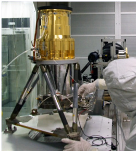
GLM FM1 sensor unit flight harness installation. Credit: LMATC
