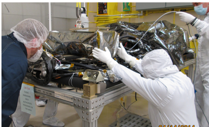
The EXIS instrument is installed on the sun-pointing platform of the GOES-R satellite. Credit: Lockheed Martin
