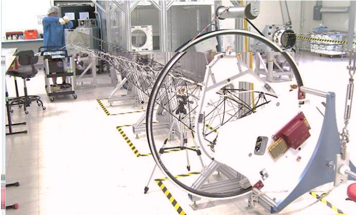
This image captures the first functional deployment of the GOES-R Magnetometer boom. Credit ATK, Goleta
