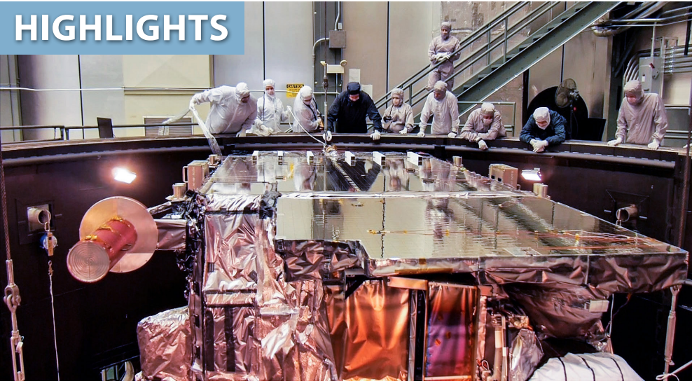
The GOES-R satellite is shown post-testing after opening thermal vacuum chamber door. Credit: Lockheed Martin
