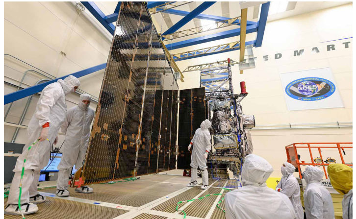
Engineers conduct the GOES-T solar array deployment test. Credit: Lockheed Martin
