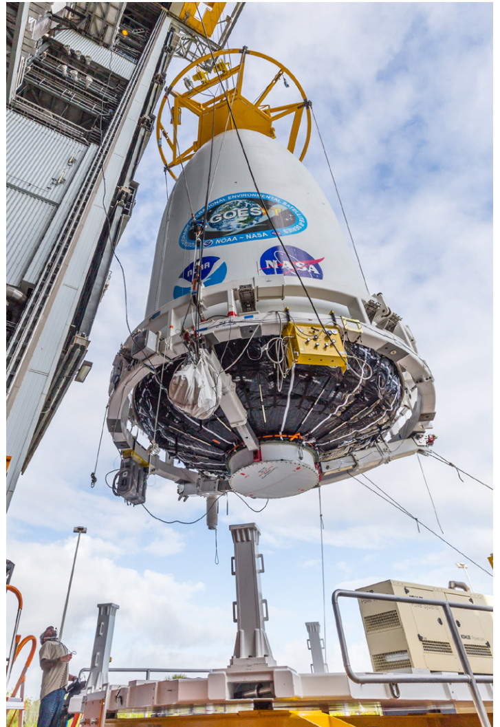
The payload fairing containing GOES-T is lifted by crane for mating to the Atlas V rocket. Photo credit: United Launch Alliance
