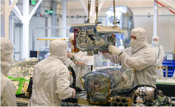
Technicians install CCOR-1 on the GOES-U solar-pointing platform. Photo credit: Lockheed Martin
