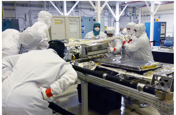
GOES-U SUVI telescope and electronics box installation. Credit: Lockheed Martin
