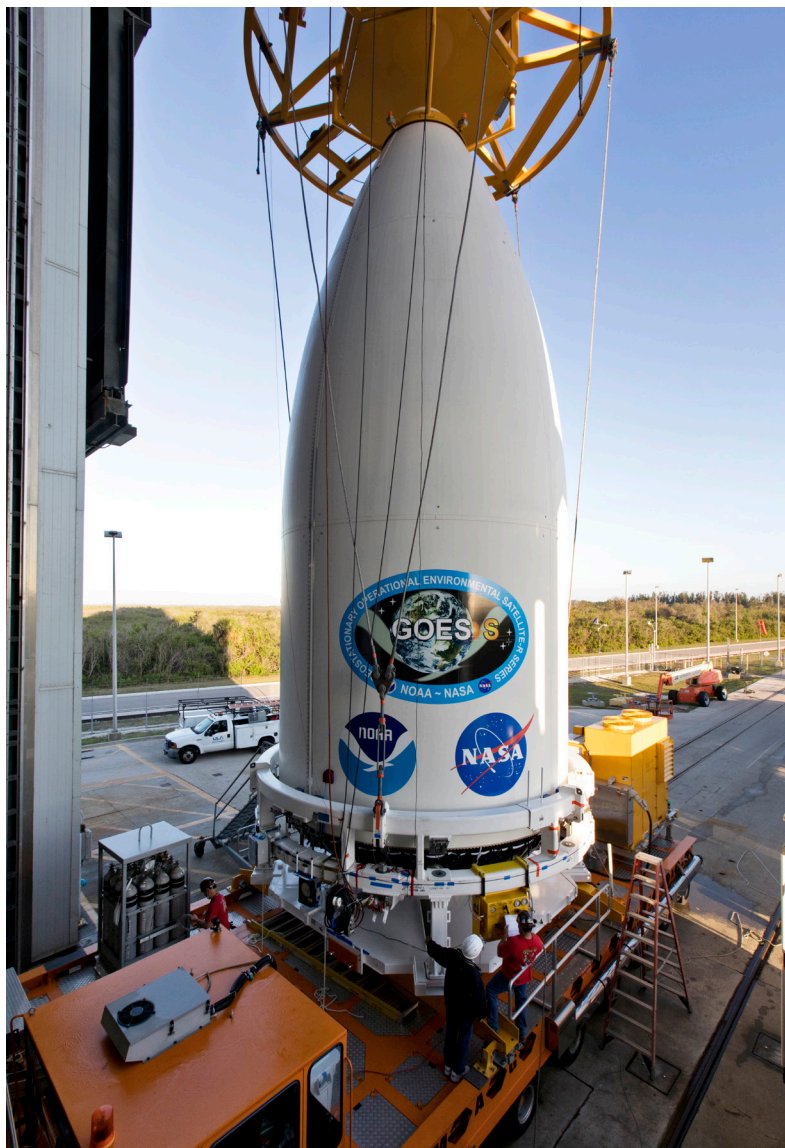
The payload fairing containing GOES-S is lifted by crane for mating to the Atlas V rocket. Credit: NASA/Glenn Benson
