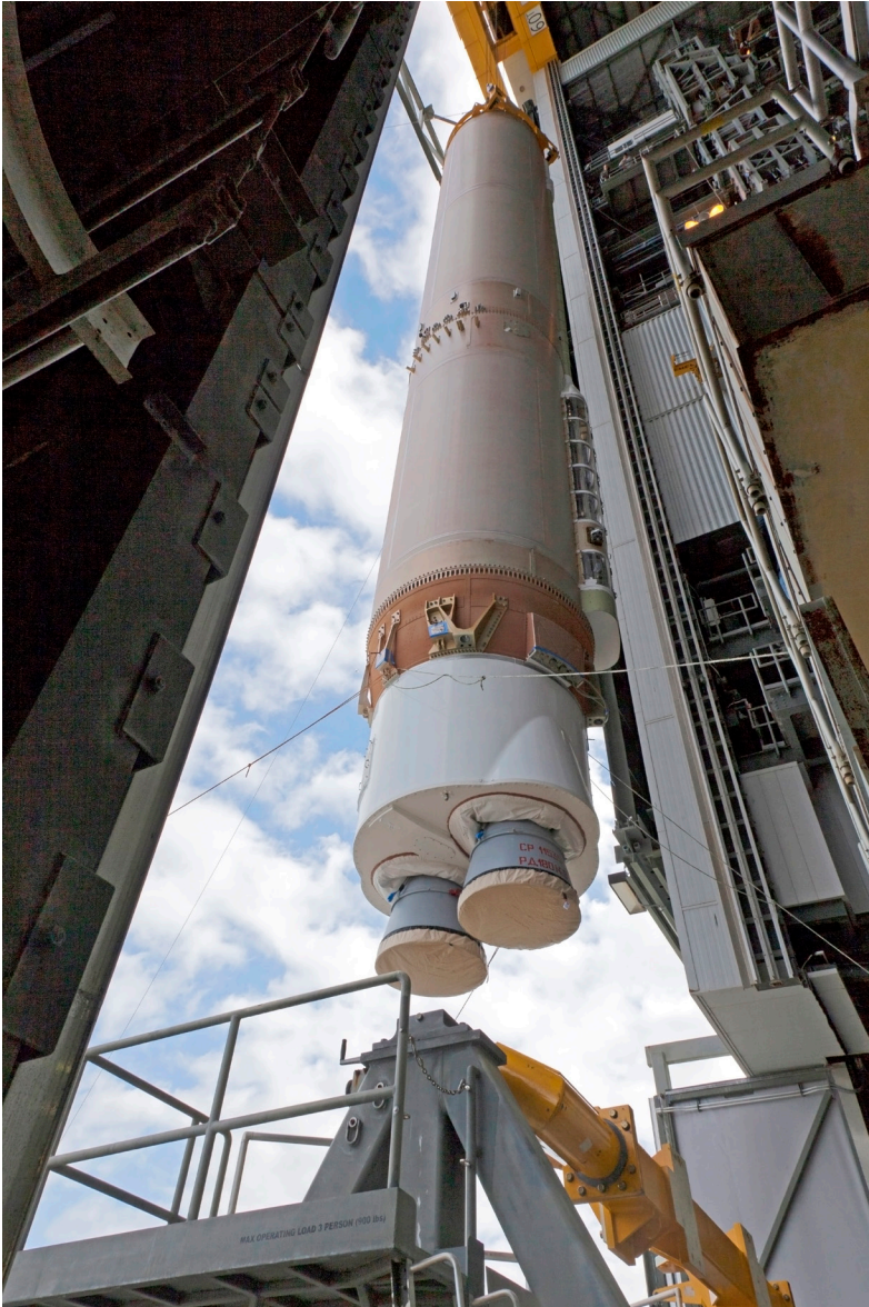
GOES-S Atlas V first stage booster lifted to vertical on stand. Credit: NASA/Ben Smegelsky
