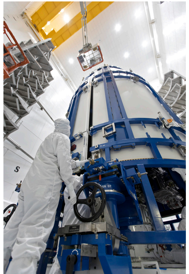
Technicians and engineers monitor progress as GOES-S is encapsulated in its payload fairing. Credit: NASA/Kim Shiflett
