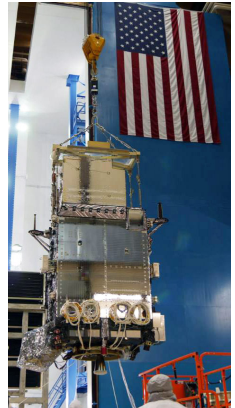
ABOVE: The GOES-R satellite is lowered into the 29' x 65' vacuum chamber where it will undergo environmental testing. RIGHT: The GOES-R satellite is transported from the clean room to the testing chamber at Lockheed Martin. Credit: Lockheed Martin
