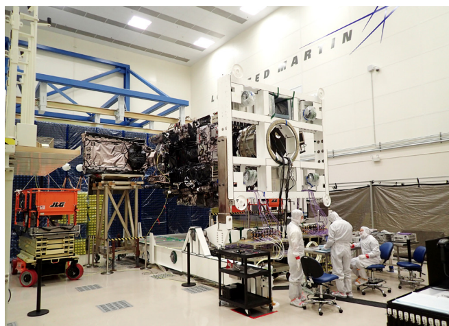
GOES-R in electromagnetic interference test configuration. Credit: Lockheed Martin
