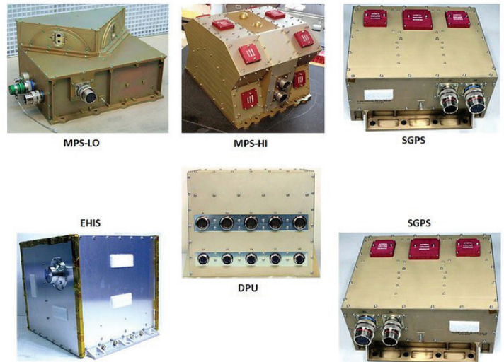
Sensors that comprise the SEISS instrument: Energetic Heavy Ion Sensor (EHIS), Magnetospheric Particle Sensors - High and Low (MPS-HI and MPS-LO), and the Solar and Galactic Proton Sensors (SGPS). Credit: Assurance Technology Corporation
