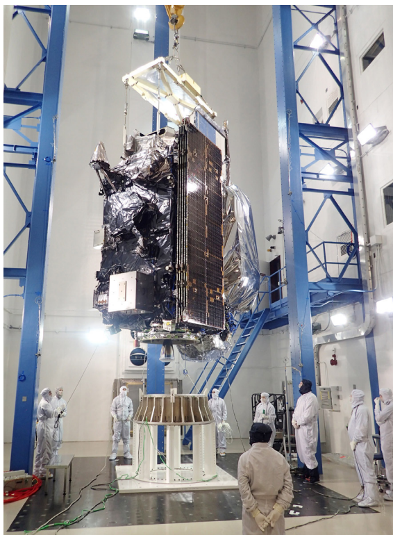
GOES-R acoustics testing. Credit: Lockheed Martin
