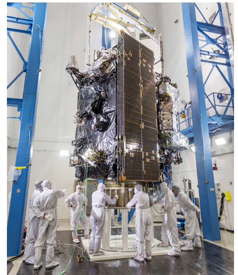
Engineers prepare GOES-S for acoustics testing in November. Credit: Lockheed Martin
