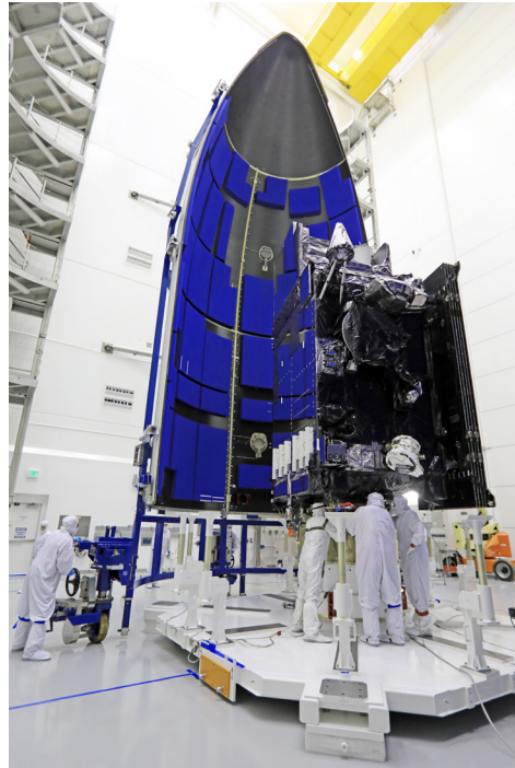
Team members with United Launch Alliance prepare GOES-R for encapsulation in the payload fairing. Credit: NASA/Kim Shiflett
