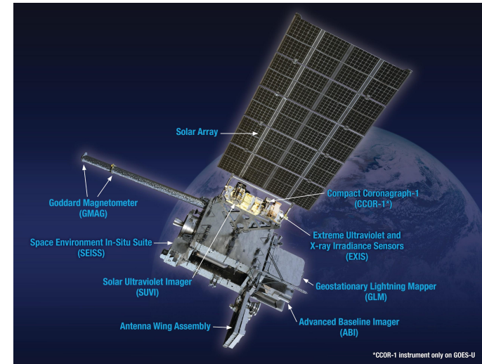
Figure 2. GOES-R Series satellites are composed of 6 (7 on GOES-U) instruments, and powered by a solar panel array.
