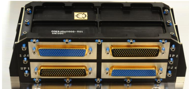
Figure 10-6. Current Sensor Unit (CSU)
