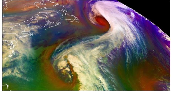
This GOES-16 air mass RGB imagery shows a pair of mid-latitude cyclones in the North Atlantic on Jan. 23, 2020. This type of imagery combines water vapor and infrared imagery and is used to monitor the evolution of cyclones and jet streaks. Credit: NOAA/CIRA
