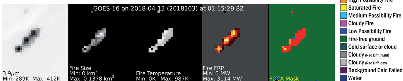
GOES-16 imagery of the Rhea Fire in Oklahoma on April 13, 2018, showing the ABI 3.9 \mu\text{m} shortwave infrared band (left column), and the various outputs of the fire detection and characterization product. From left: fire size, fire temperature, and fire mask. Fire radiative power is shown in colors from black to red for 0 to 1000 megawatts (MW), red to yellow for 1000 to 2000 MW, and yellow to white for 2000-3000 MW. Credit: CIMSS
