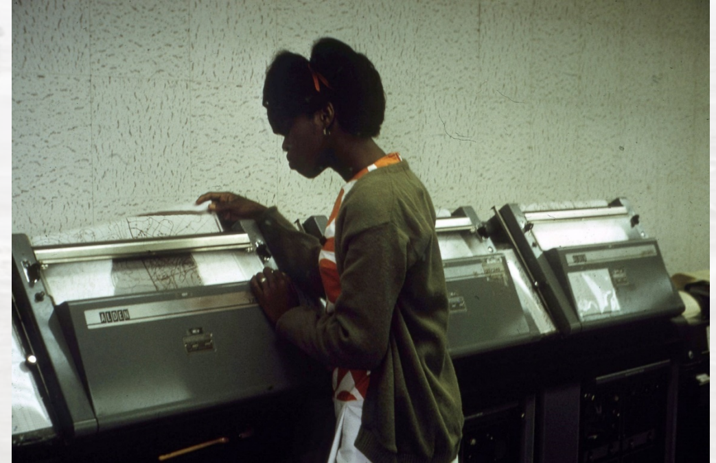
Facsimile weather maps and satellite composites were received via phone line, circa 1971
