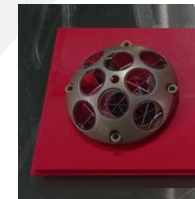
LRA(Laser Retroreflector Array) provided by NASA. The LRA consists of an array of multiple mirrors that are retroreflective and reflect light back in the direction of origin. Mass is approximately 21g.
