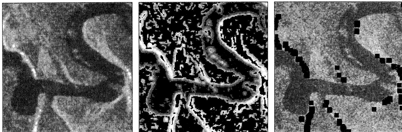
Figure 2: Preprocessing products: Kuan-filtered SAR image (left), preclassified image (mid), strong scatterers (right).
