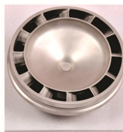
3D printed proto-type realized in 718 alloy
