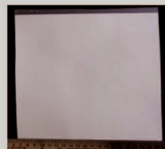
Typical green tape (6.5" square) for IC package and sintered thin sheet(150 \mu ) for MIC substrate (courtesy: NAL)
