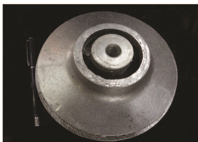
Aluminum alloy Impeller made through investment casting process
