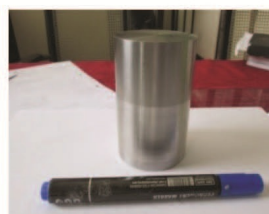
Diffusion bonded commercially pure (CP)-70 titanium alloy and stainless steel rod
