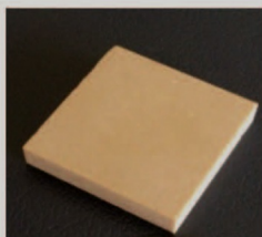
Sintered substrate (28×28×2.5mm) for HMC
