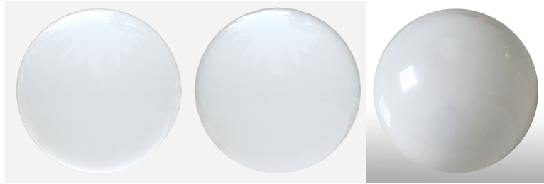
Figure 7. Close up of a smooth plastic ball. Single scattering model (left), multiple scattering model (center), and reference photograph (right).
