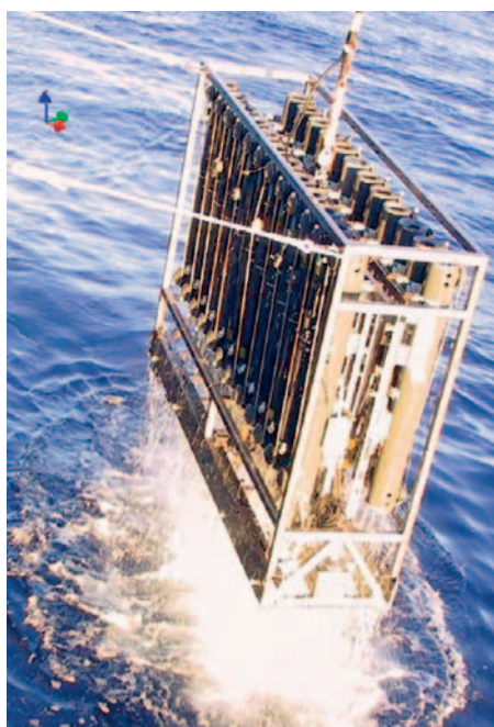
An ultraclean sampler for trace metals in seawater emerges from the ocean. © NIOZ
