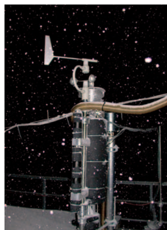
Counterflow virtual impactor inlet system at the Jungfrauoch research site.
