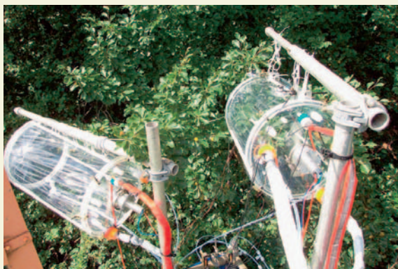
Two cuvettes (stabilised Teflon film bags), one is an empty reference, the other one is enclosing a branch to investigate trace gas exchange between plants and the atmosphere.
