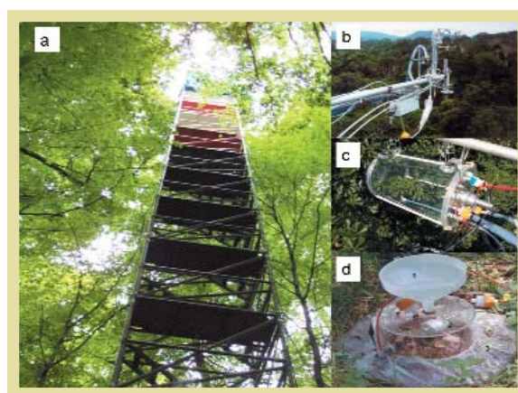
A large tower (a) reaching above the canopy top (by more than 10 m) provides access to measure turbulent transport above the forest (by sonic anemometer (b)) and allows to place enclosures (cuvettes) around a leaf or branch (c). At the forest floor, soil chambers (d) are used to study soil gas exchange.
