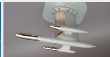
The air inlet system.
