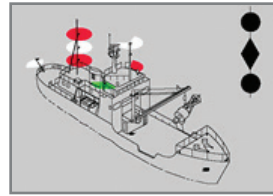
Vessel Restricted in Her Ability to Maneuver— Making way; less than 50 meters in length
