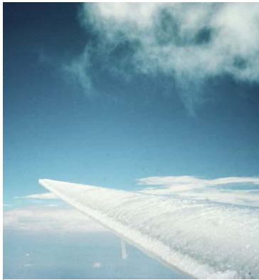
Icing buildup on the wing of a small aircraft Image credit UCAR.
