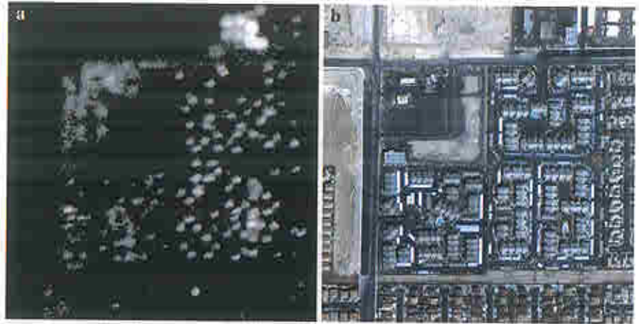
Fig. 1 (a) Nighttime lights observed for a section of Las Vegas, Nevada at 1.5 m resolution. The image has been co-registered to the Ikonos image shown in (b). (b) True color Ikonos imagery for a section of Las Vegas, Nevada
