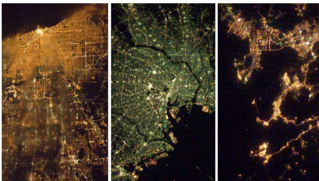
Figure 2. Color camera images of Chicago, Tokyo and Hong Kong acquired at sixty meter resolution from the International Space Station. Note the presence of optically thin clouds in the Chicago image, resulting in a blur of the street pattern.
