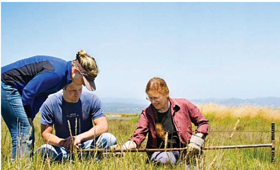
Figure 3-1. Lori Dengler and her students examine a sediment core taken from Humboldt Bay, California. Cores reveal evidence of centuries of earthquake and tsunami activity and allow tsunami scientists to estimate recurrence intervals of Cascadia subduction zone earthquakes in the Humboldt Bay region. (Photo credit: Kellie Jo Brown, Humboldt Bay University.)
