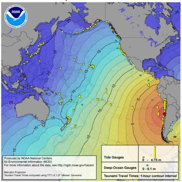
September 16, 2015 tsunami water heights tide gauges, and DARTs; and estimated tsunami travel times plotted at 1-hour intervals (black lines) using the earthquake epicenter (star) as a point source. The maximum amplitude was 4.75 meters at Coquimbo, Chile. (Credit: J. Varner, NCEI)
