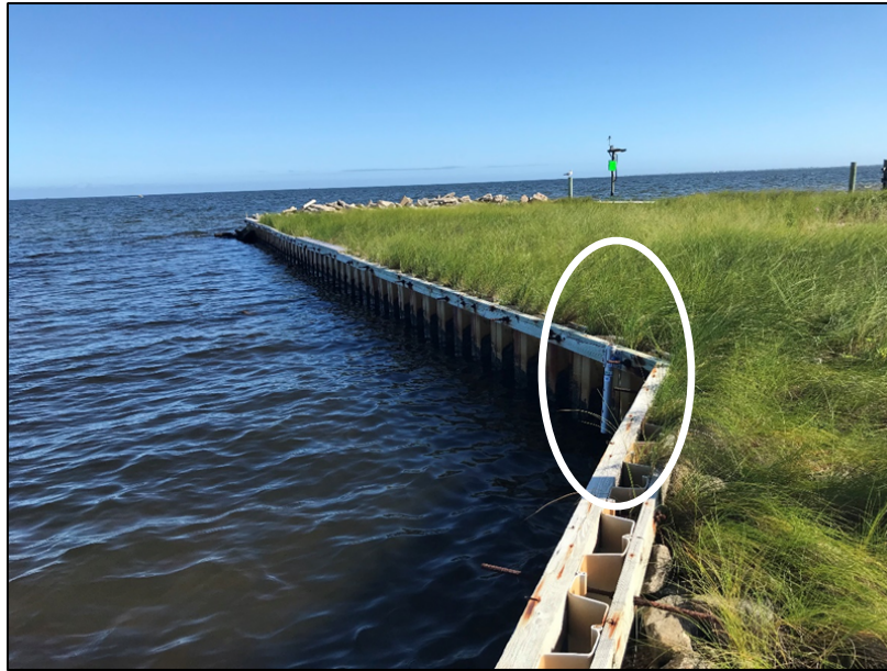
Figure 8. (a) A USGS pressure sensor installed on a bulkhead on Pamlico Sound in Buxton, NC (highlighted by the white ellipse). (b) Instantaneous water level (gray, ft above NAVD88), wave-filtered water level (blue, ft above NAVD88) and barometric pressure (red, in Hg) recorded from the sensor. Images courtesy of the USGS.
