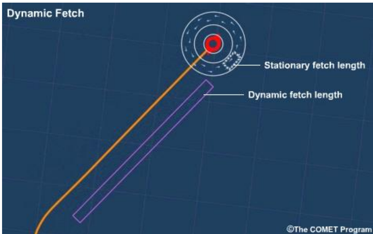
Figure 14: Dynamic Fetch Diagram. Wind direction and storm direction are the same on the right side of a northern hemisphere storm. If the storm direction is fairly straight and the speed isn't too fast or too slow, the wave generation area can travel with the storm, increasing wave heights well above what the stationary fetch length of the storm can produce.
