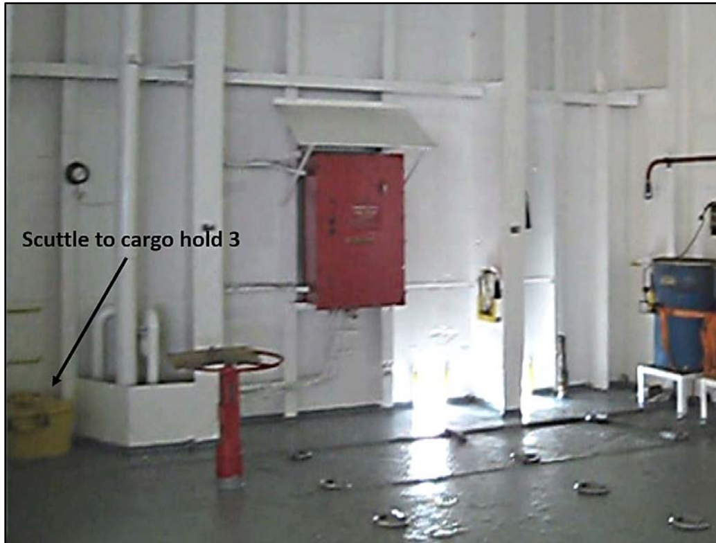
Figure 57. Second deck scuttle to hold 3. (Photo by former El Faro second mate)
