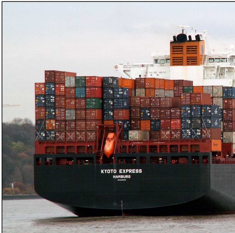
Figure 55. Stern-launched freefall lifeboat on large container ship. Orange lifeboat is shown in launch position amid stacks of containers. (Photo by Sascha Heuer; used by permission)
