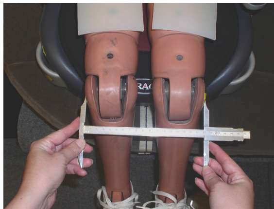
Figure 35. Setting the distance between the outer edges of the knees to 180 mm for the 6-year-old and 220 mm for the 10-year-old.
