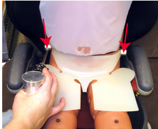
Figure 25 Checking that the X and Z values of the symmetrical points
