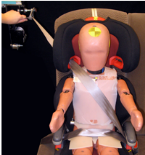
Figure 41. Feeding the shoulder belt into the retractor
