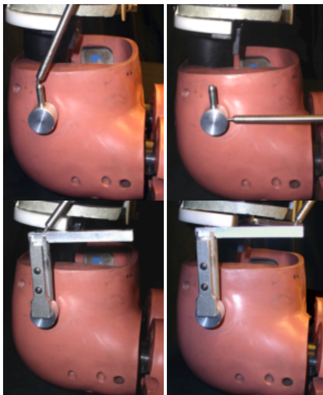
Figure 8. Digitizing the reference marks on the hip offset tools with the upright attachment on and off.
