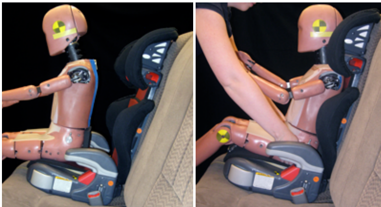
Figure 22. Moving the ATD rearward in the seat
