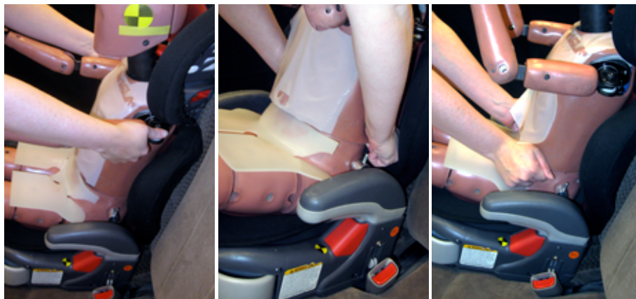
Figure 27. Pushing clavicles down and rearward at shoulder with arms out and then pulling jacket down
