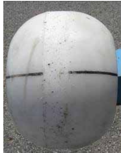
Figure 5.7: Wear after 14 strikes between wheel and test surface. Diameter change is estimated at \sim 1/32 inch or less.
