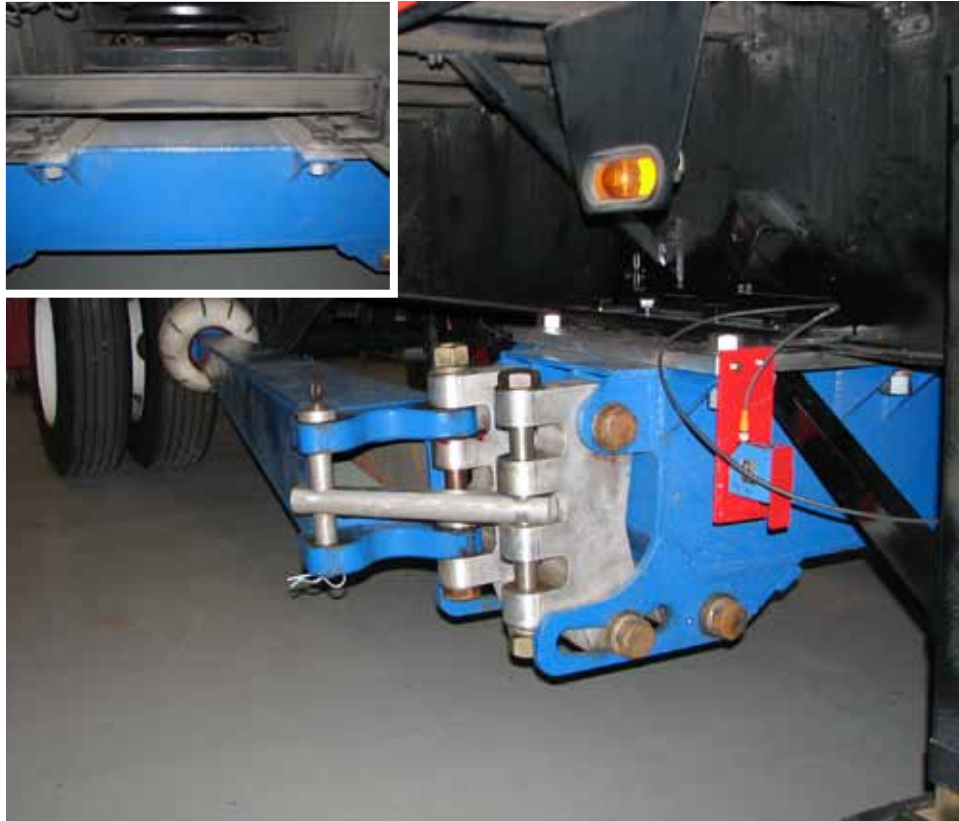
Figure 5.1: Center: shows the main beam of the new outriggers mounted to a 28ft. flatbed type trailer. The main trailer rails are clamped on the outside and inside Upper Left: Shows the inside flanges of the trailer main rails were clamped and bolted to the outrigger adapter plate.
