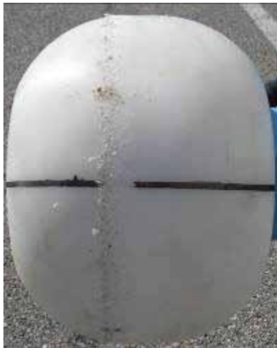
Figure 5.5: Wear after the first observed contact between wheel and test surface.
