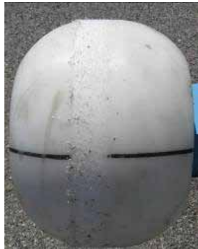
Figure 5.6: Wear after seven strikes between wheel and test surface.
