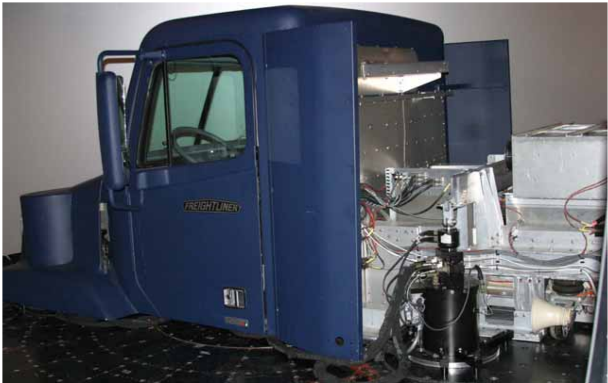
Figure 2.4 - Truck cab showing vertical actuator for vibration cues
