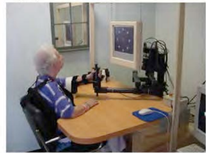
Figure 1 Stroke Inpatient during Therapy at the Burke Rehabilitation Hospital (White Plains, NY). Therapy is being conducted with a commercial version of MIT-MANUS (Interactive Motion Technologies, Inc., Cambridge, MA).
