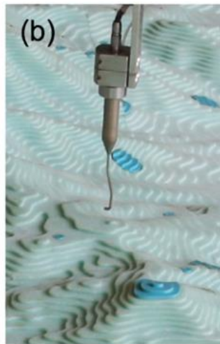
(a) Cobra Probe installed in instrument traverse
