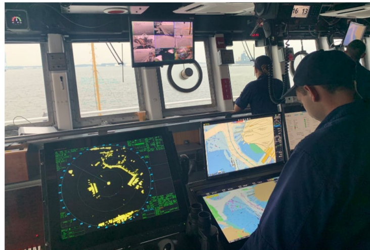
Electronic navigational chart displayed on an Electronic Chart Display and Information System (ECDIS) on NOAA Ship Thomas Jefferson. Photo credit: NOAA
