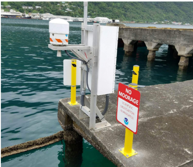
An NWLON station was installed in American Samoa at the Port of Pago Pago. The station provided NOAA's Tsunami Warning Center with critical tsunami data from the Tonga volcanic eruption in January to help warn local communities and Pacific Island governments.
