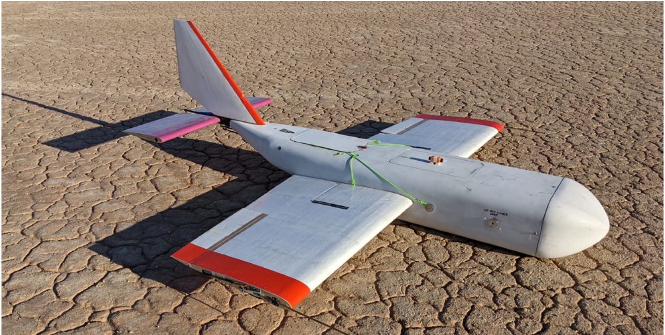
NOAA's new uncrewed glider called, "High-altitude Operational Return Unmanned System (HORUS)" poised to help vastly increase high-altitude research.
